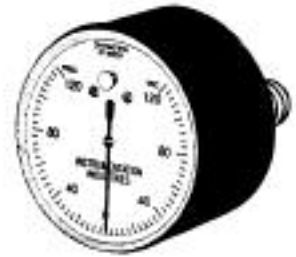
#GZ-NS120-TRS Gauge reads \pm 120\text{cm H}_2\text{O} in 4cm dial markings with 1/4" NPT connection in rear.
