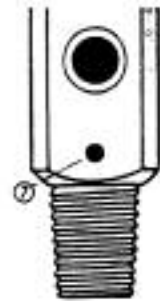
CGA Connection No. 965 Medical Cylinder Valve Connection N 2 O & O 2 mix (N 2 O 47.5 to 52.5%)
